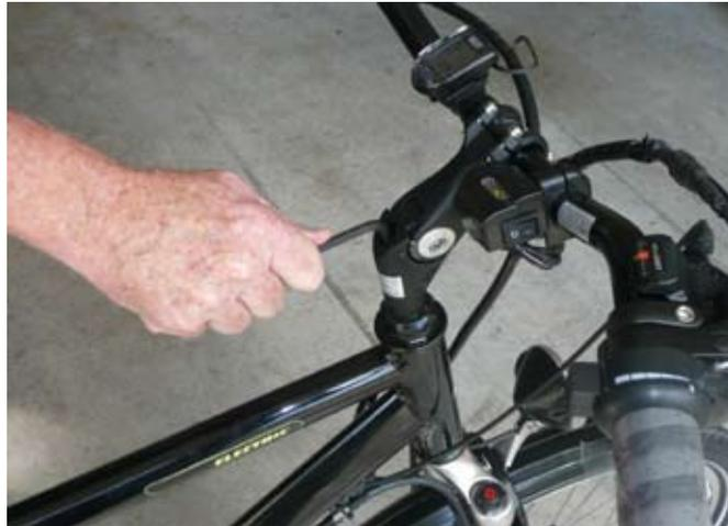
3. Turn the handlebar to the desired angle and tighten using the 4mm wrench.
