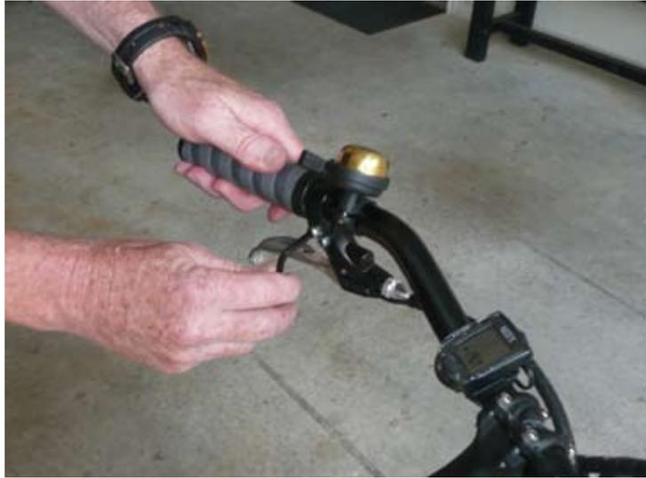
5. If needed, adjust and tighten the battery meter with slotted head screwdriver.
