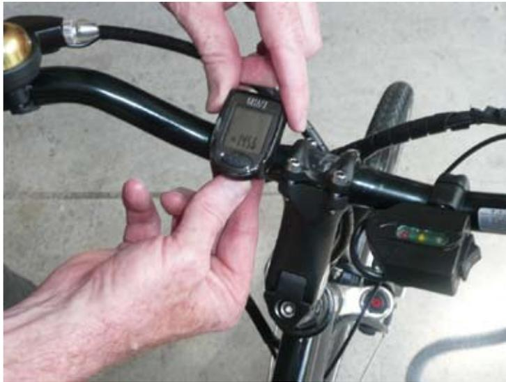
b. Press the front button and using a pencil or pen, press the gray button on the back.
