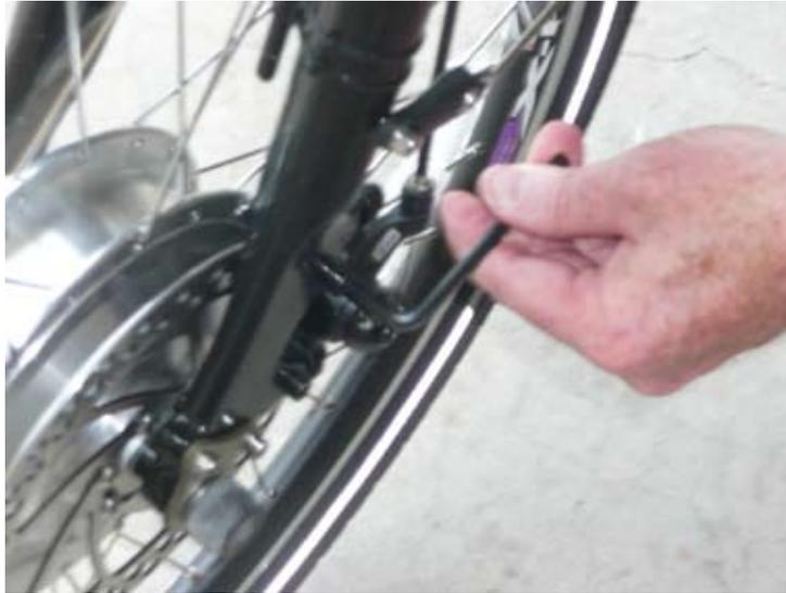
9. If you wish to change the angle of the front stem, you can adjust it by loosening the adjustment screw with a 5mm wrench, and re-tighten after adjustment.
